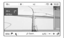
If the autozoom function is activated (AUTO is displayed below the map view), the zoom level changes automatically when approaching a turning manoeuvre during active route guidance. This way, you always get a good overview of the respective manoeuvre.
