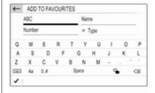
Keyboards for text input may contain several input fields. To enable a field for text input, touch it.
