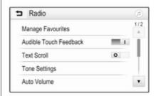
Touch the screen button next to **Audible Touch Feedback** to activate or deactivate the function.
