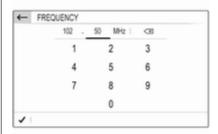
Keyboards for number input may contain several input fields. In the illustrated example, you first need to touch the input field behind the decimal point, before you can enter the decimal digits.
