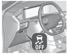
ESC and Anti-Slip Regulator (ASR) system can be deactivated if it is required: press .
