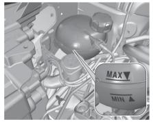
If the coolant level is at the MIN mark or below, seek the assistance of a workshop to have the engine coolant topped up.
