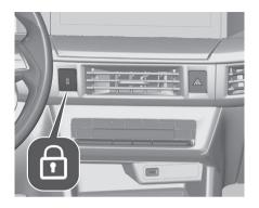
Press to lock. The LED in the button illuminates.
