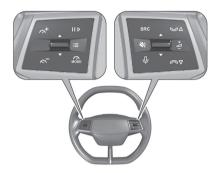
The cluster menu, some driver assistance systems, the Infotainment system and a connected mobile phone can be operated via the controls on the steering wheel.
