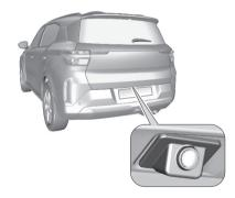
The rear view camera assists the driver when reversing by displaying a view of the area behind the vehicle. It allows views of the vehicle's surroundings to be
