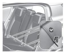
Fasten vehicle-approved ISOFIX child restraint systems to the ISOFIX brackets. Specific vehicle ISOFIX child restraint system positions are marked in the child restraints table.
