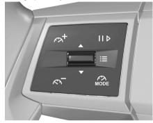
If the system is active, the preset speed can be changed by pressing  $^{\dagger}$ to
