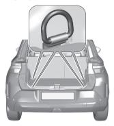
The lashing eyes are designed to secure items against slippage, e.g. using lashing straps or luggage net.
