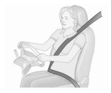
The seat belts are locked during heavy acceleration or deceleration of the vehicle, holding the occupants in the seat position. Therefore the risk of injury is considerably reduced.
