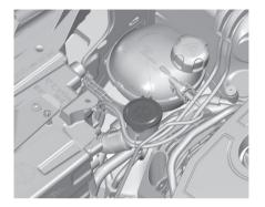
Fill with clean water mixed with a suitable quantity of approved windscreen washer fluid that contains antifreeze.
