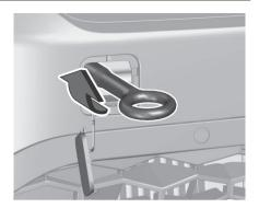
Screw in the towing eye as far as it will go, until it stops in a horizontal position. Attach the tow rod to the towing eye. The towing eye must only be used for towing and not for recovering the vehicle. Switch on ignition to release steering wheel lock and to permit operation of brake lights, horn and windscreen wiper.
