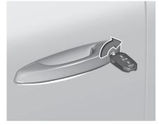
Manually lock the left front door by inserting and turning the key in the lock cylinder. With working central locking system the vehicle will be locked.
