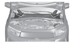
The air intake in front of the windscreen in the engine compartment must be kept clear to allow air intake. Remove any leaves, dirt or snow.
