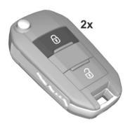
Press on the radio remote control twice within five seconds.
