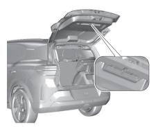
Stow the warning triangle in the space at the rear of the tailgate and secure it with the Velcro® fastener.
