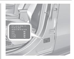
The tyre pressure information label on the left or right door frame indicates the original equipment tyres and the corresponding tyre pressures. The tyre pressure data refers to cold tyres. It applies to summer and winter tyres.
