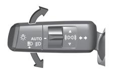
When the vehicle is parked, the parking lights on one side can be activated:
