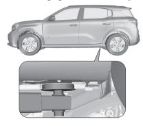
The rear arm position of the lifting platform is centrically under the relevant vehicle jacking point.
