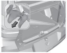
The bag with the coupling ball bar is stowed on the rear floor cover in the load compartment.
