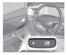
Press the button to deactivate the rear door power windows; the LED illuminates. To activate, press again.
