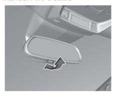
To reduce dazzle, pull the lever on the underside of the mirror housing.
