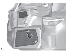
Open the tailgate then unclip the access cover on the relevant side.
