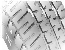
The legally permissible minimum tread depth (1.6 mm) has been reached when the tread has worn down as far as one of the tread wear indicators (TWI). Their
