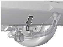
Attach the breakaway stopping cable to eye.
