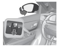
Move the switch to the centre position. Pull it rearwards. Both exterior mirrors are folded.
