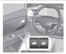
Operate for the respective window by pushing to open or pulling to close. Long pushing or pulling: the window moves up or down completely when the switch is released.
