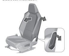
Push the lever backwards. Lean on the backrest to obtain the desired angle.
