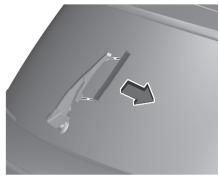
Lift wiper arm. Disengage wiper blade as shown in illustration and remove. Attach the wiper blade slightly angled to the wiper arm and push until it engages. Lower wiper arm carefully.
