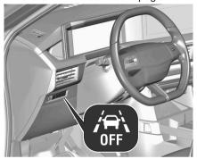
If the system is activated, the LED in the button is not illuminated. To activate the system when the system is deactivated, press the button.
