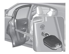
Turn the red child lock in the rear doors to the horizontal position by using a key. The door cannot be opened from the inside.
