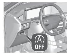
The system is ready to operate when the LED in the button is not illuminated. To activate the system when the system is deactivated, press (A).
