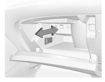
Move the slider back or forth in order to enable or disable glovebox cooling.
