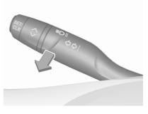
Pull to activate the headlight flash. Pull to deactivate high beam.
