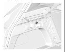
At the left sidewall in the load compartment, another 12 V power outlet is located.
