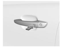
Electronic key system: Unlocking the vehicle by pressing on one of the front door handles at the markings deactivates the anti-theft alarm system.
