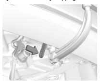
Attach breakaway stopping cable to eye.
