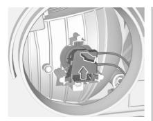
Press retaining clip upwards and pull the bulb socket toward the rear.
