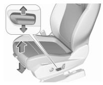
Move switch upwards / downwards.
