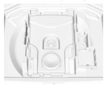
The towing eye and the chocks are located in a box below the floor cover in the load compartment.
