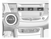
Press **MENU** to enter the menu. Select **Temperature conditioning**. Select heating or ventilation. Define a timer.
