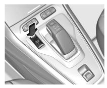
The drive modes can be selected via the drive mode selector. The selected drive mode is indicated in the Driver Information Centre and in the Driver Info Display. Selecting a drive mode is only possible if **READY** is displayed in the instrument cluster.
