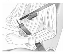
Withdraw the seat belt from the retractor, guide it untwisted across the body and insert the latch plate into
