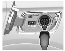
Plug in the vehicle plug of the charge cord into the charge port on the vehicle.
