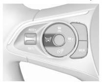
Press of, the adaptive cruise control is in pause mode and a message is displayed. The vehicle is driven without adaptive cruise control.
