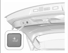
Press button \*#" in the open tailgate, the whole vehicle will be locked after hands-free closing of the tailgate.
