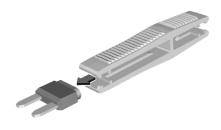
Grab the fuse with the fuse extractor and withdraw the fuse.
