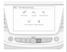
Press **SET** to open settings menu. Use touch buttons to operate the display.
