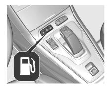
Press . After depressurisation the fuel filler flap is unlocked. This can take up to one minute.
