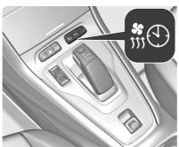
The operating status of the parking heater is shown by an indicator with a LED.
