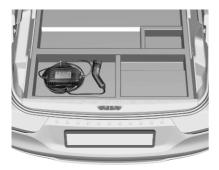
A portable charge cord used to charge the vehicle high voltage battery is stored under the rear floor storage cover in the load compartment \$\Delta\$ 194. The charge cord is compatible with the domestic electrical outlet of the respective country. It includes a control box with charging status indicators.
