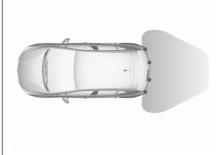
The system operates with ultrasonic parking sensors in the rear bumper.
