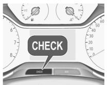
To retrieve the status of the service information at any time press button **CHECK**. The service information is displayed for a few seconds.
