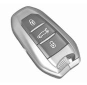
The central locking system can also be operated with the buttons on the electronic key.
