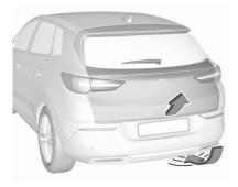
To open or close the tailgate move the foot below the rear bumper back and forth in the area below the number plate. Do not hold the foot longer or move too slow below the bumper. The electronic key must be outside the vehicle, within a range of approx.
