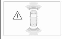
Additionally, the distance to rear and front obstacles is displayed by changing distance lines in the Info Display № 102.
