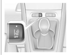
After ignition is switched on, the lane departure warning system is activated. If the system is activated, the LED in the button \( \mathbb{I} \) is not illuminated. To activate the system when the system is deactivated, press \( \mathbb{I} \).
