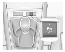
The system is ready to operate when the LED in the parking assist button is not illuminated.
