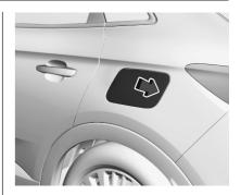
Push the rearward edge of the charge port door in and release to open the door.
