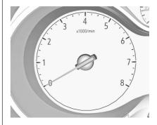
Displays the engine speed.
