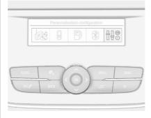
Press **MENU** to open the menu page. Use four-way button to operate the display:
