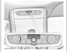
Adjust the air flow by turning rotary ring to the desired speed. Turn anticlockwise to decrease or turn clockwise to increase. Fan speed can also be changed in the climate settings menu. Press **MENU** to enter the menu.
