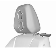
Press release button, adjust height, engage.
