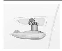
Turn bulb socket clockwise and remove from light assembly.
