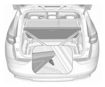
To hold the load compartment cover in an upright positon, lift it up past the retractable stops.
