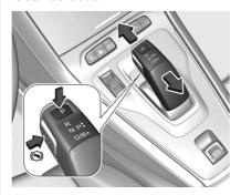
P: park position, front wheels are locked, engage only when the vehicle is stationary and the parking brake is applied
