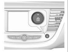
This function can be activated or deactivated at any time. With the ignition on, press \( \text{\text{d}} \) until an audible signal starts and a corresponding message is displayed.
