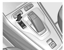
All-wheel drive mode can be activated using the driving mode switch. Activation is shown in the Driver Information Centre and the Info Display.
