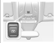
Press gently to the first detent at the rear: the sunblind is opened as long as the switch is operated.
