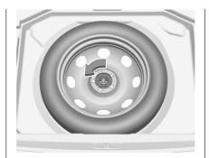
The spare wheel is located in the load compartment beneath the floor covering.
