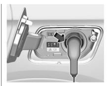
The start of charging is indicated by the green flashing of the status indicator at the charge port and at the control box of the charge chord.
