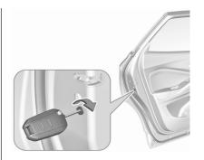
To lock the other doors, remove the black cover by using a key.
