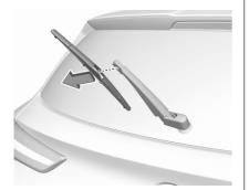
Lift wiper arm. Disengage wiper blade as shown in illustration and remove.
