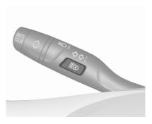
Activate the high beam assist by pressing \$\exists\$0. The LED of the button illuminates if the high beam assist is activated. High beam is switched on automatically at a speed above 15 mph. High beam is switched off at a speed below 9 mph, but high beam assist remains active.
