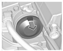
1. Remove the protective cover by pulling.
