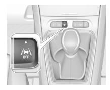
If the system is activated, the LED in the button as is not illuminated. To activate the system when the system is deactivated, press as.
