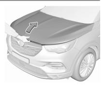
Push the safety catch upwards and open the bonnet.
