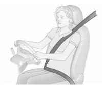
Pull out the seat belt and fasten in seat belt buckle. The seat belt must not be twisted and must fit close against the body. The backrest must not be tilted back too far (maximum approx. 25°).
