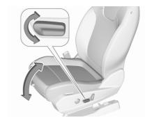
Move front of switch upwards / downwards.
