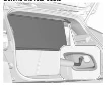
There are installation openings on both sides in the roof frame above the rear seats: suspend and engage rod of net at one side, compress rod and suspend and engage at the other side.
