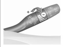
Turn the adjuster wheel to adjust the sensitivity.
