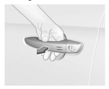
Pass a hand behind the door handle of a front door to unlock the vehicle or press the tailgate button.
