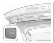
To close, press in the open tailgate until the tailgate starts to move.
