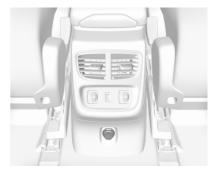
A 12 V power outlets is also located in the rear console.
