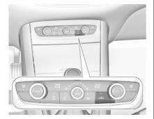
Press \$\sigma\$ to activate the air recirculation mode. The LED in the button illuminates to indicate activation.
