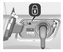
Once charging, the vehicle plug will be locked to the charge port and cannot be disconnected while charging is active. (1) indicator illuminates.
