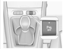
The system is switched off when reverse gear is disengaged. Press to deactivate the system manually. The LED in the button illuminates when the system is deactivated. If the system has been deactivated manually, it is not reactivated automatically the next time the ignition is switched on.
