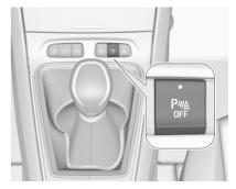
The system is switched off when reverse gear is disengaged. Press to deactivate the system manually. The LED in the button illuminates when the system is deactivated. If the system has been deactivated manually, it is not reactivated automatically the next time the ignition is switched on.
