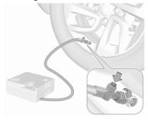
16. Continue driving immediately so that sealant is evenly distributed in the tyre. After driving approx. 3 miles but no more than 10 minutes, stop and check tyre pressure. Screw compressor air hose directly onto tyre valve when doing this. Fill tyre as described
