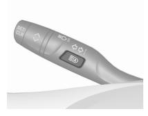
Activate the high beam assist by pressing **■**. The LED of the button illuminates if the high beam assist is activated. High beam is switched on automatically at a speed above
