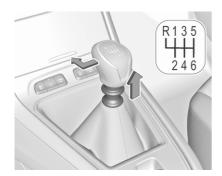
To engage reverse on 6-speed transmission, depress the clutch pedal, pull the ring under the selector lever and move the selector lever quite to the left and front.
