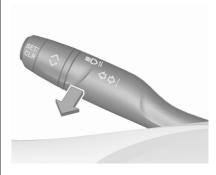
Pull to activate the headlight flash. Pull to deactivate high beam.
