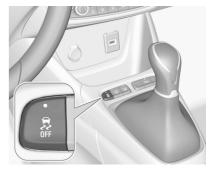
ESC and traction control system can be deactivated, everytime it is required: press #.
