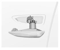
2. Turn bulb socket clockwise and remove from light assembly.
