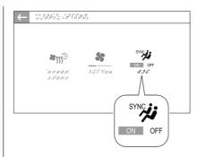
Set \*\*\*\* to **ON** to link passenger side temperature setting to the driver side Touch MONO or SYNC to link passenger side temperature setting to the driver side.
