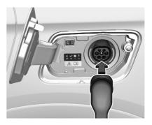
Plug in the vehicle plug of the charging cable into the charging port on the vehicle.
