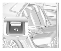
Fasten vehicle-approved ISOFIX child restraint systems to the ISOFIX brackets. Specific vehicle ISOFIX child restraint system positions are marked in the ISOFIX table ♀ 64.
