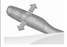
Push to switch from low to high beam.
