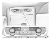
Set the preselected temperatures separately for the driver and the front passenger to the desired value using the left and right rotary ring. The rotary ring on the passenger side changes the temperature of the passenger side. The rotary ring on the driver's side changes the temperature of the driver's side or of both sides, depending on activation of synchronisation MONO in the climate control settings menu. Press MENU to enter the climate control settings menu.
