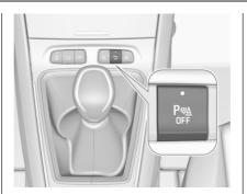
The system is ready to operate when the LED in the parking assist button is not illuminated.
