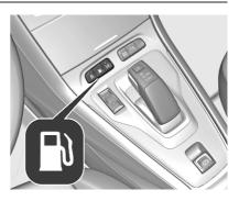
Press : After depressurisation the fuel filler flap is unlocked and bounces a bit.
