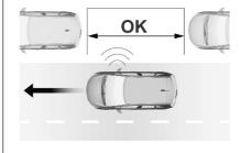
When a free slot is detected, a visual feedback on the Info Display and an acoustic signal are given. Stop the vehicle, select reverse gear, release the steering wheel and start moving without exceeding 4 mph.
