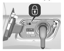
Once charging, the vehicle plug will be locked to the charging port and cannot be disconnected while charging is active. (1) indicator illuminates
