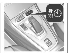
The operating status of the parking heater is shown by a LED.
