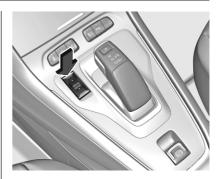
All-wheel drive mode can be activated using the driving mode switch. Activation is shown in the Driver Information Centre and the Info Display.
