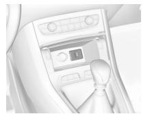
A USB port is located behind the storage cover. Press cover to open.
