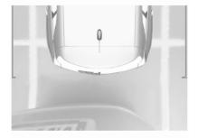
The camera records the vehicle's surroundings during the manoeuvre in order to reconstruct a view from above the rear or the front of the vehicle in its near surroundings. Thus, the vehicle can be manoeuvred around obstacles nearby. This view is available with auto mode or in the view selection menu.
