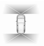
The 180° view facilitates reversing out of a parking bay, making it possible to see the approach of vehicles, pedestrians and cyclists. This view is not recommended for carrying out a complete manoeuvre. It is made up of three areas: left 1, centre 2 and right 3. This view is available from the view selection menu only.
