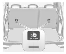
In addition to the ISOFIX brackets, fasten the Top-tether strap to the Top-tether anchors.
