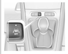
If the system is activated, the LED in the button # is not illuminated. To activate the system when the system is deactivated, press #.
