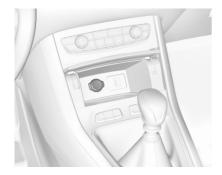
A 12 V power outlet is located behind the storage cover. Press cover to open.
