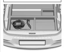
A portable charging cable used to charge the vehicle high voltage battery is stored under the rear floor storage cover in the load compartment
