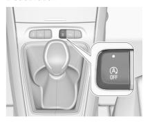
Deactivate the stop-start system manually by pressing @. The deactivation is indicated when the LED in the button illuminates.
