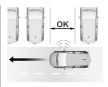
When a free slot is detected, a visual feedback on the Info Display and a first acoustic signal are given. Drive slowly forwards. When the second acoustic signal is given, stop the vehicle, select reverse gear, release the steering wheel and start moving slowly. A visual feedback is given on the Info Display.
