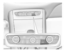
Press \$\simes \text{ to activate the air recirculation mode. The LED in the button illuminates to indicate activation.}
