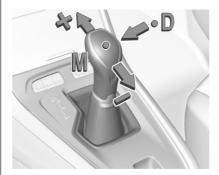
Move selector lever out of position  ${\bf D}$  towards the left in position  ${\bf M}$ .
