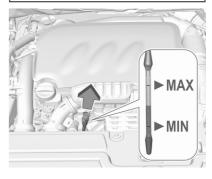
Pull out the dipstick, wipe it clean, reinsert it fully, pull out and read the engine oil level.
