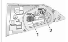
Turn the bulb socket anticlockwise and remove it from the light assembly. 7. Detach the bulb from the bulb socket and replace the bulb:
