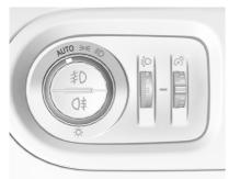
When the automatic light control function is switched on and the engine is running, the system switches between daytime running lights and headlights automatically depending on the external lighting conditions and information given by the wiper system.
