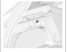
At the left sidewall in the load compartment, another 12 V power outlet is located.
