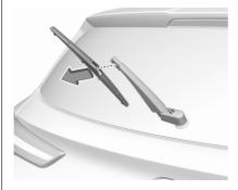
Lift wiper arm. Disengage wiper blade as shown in illustration and remove.
