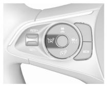
Press 'n', the adaptive cruise control is in pause mode and a message is displayed. The vehicle is driven without adaptive cruise control.
