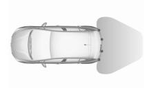
The system operates with ultrasonic parking sensors in the rear bumper.
