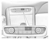
Press so to activate air recirculation mode. The LFD in the button. illuminates to indicate activation.
