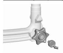
Remove the cover from the lock of the rotary knob and verify whether the rotary knob is locked. If the rotary knob cannot be turned, it is locked.
