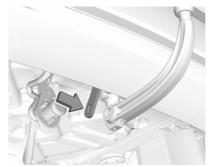
Attach breakaway stopping cable to eye.
