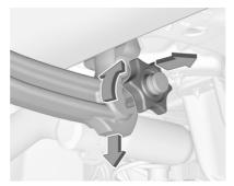
Open the protective flap and turn the key to position  $\widehat{\exists}$  to unlock the coupling ball bar.
