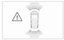
Additionally, the distance to rear and front obstacles is displayed by changing distance lines in the Info Display \$\frac{100}{2}\$.
