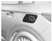
2. Push the rearward edge of the charging port flap in and release to open the flap.
