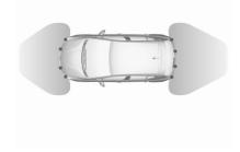
The system operates with ultrasonic parking sensors in the rear and front bumper.
