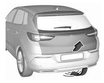
To open or close the tailgate move the foot below the rear bumper back and forth in the area below the number plate. Do not hold the foot longer or move too slow below the bumper. The electronic key must be outside the vehicle, within a range of approx. 1 m of the tailgate.
