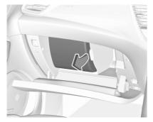
In right-hand drive vehicles, the fuse box is located behind a cover in the glovebox. Open the glovebox and remove the cover. Depending on the version, different instrument panel fuse boxes are available:
