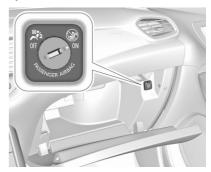
The front passenger airbag system can be deactivated via a keyoperated switch in the glovebox. Use the ignition key to choose the position:
