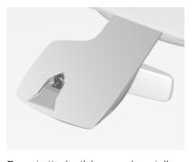
Do not attach stickers such as toll road stickers or similar on the windscreen in the area of the interior mirror. Keep the sensor free from dust, dirt and ice. Otherwise the detection zone of the rain sensor / light sensor and the view area of the camera in the mirror housing could be restricted.
