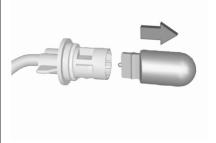
3. Detach the bulb from the bulb socket and replace the bulb.
