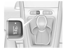
After ignition is switched on, the lane departure warning system is activated. If the system is activated, the LED in the button is not illuminated. To activate the system when the system is deactivated, press is.
