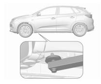
Front arm position of the lifting platform centrically under the relevant vehicle jacking point.
