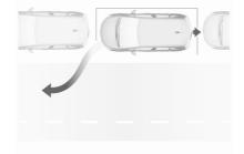
Move forwards and backwards while observing the warnings of the Parking assist until the end of manoeuvre is indicated. The manoeuvre is complete when the vehicle's front wheels are out of the parking slot.
