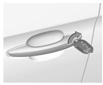
Manually lock the left front door by inserting and turning the key in the lock cylinder.
