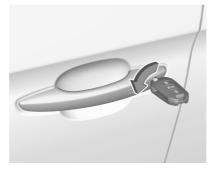
Manually unlock the left front door by inserting and turning the key in the lock cylinder.
