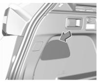
1. Open the tailgate then unclip the access cover on the relevant side.
