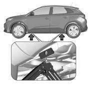
3. Ensure the jack is correctly positioned under the relevant vehicle jacking point.
