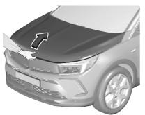
Push the safety catch upwards and open the bonnet.
