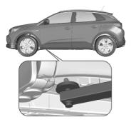
Front arm position of the lifting platform centrically under the relevant vehicle jacking point.
