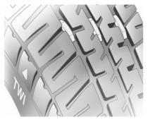
The legally permissible minimum tread depth (1.6 mm) has been reached when the tread has worn down as far as one of the tread wear indicators (TWI). Their position is indicated by markings on the sidewall. If there is more wear at the front than the rear, swap round front wheels and rear wheels periodically. Ensure that the direction of rotation of the wheels remains the same.
