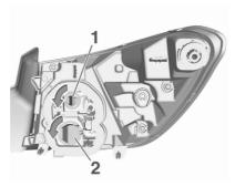
7. Detach the bulb from the bulb socket and replace the bulb.
