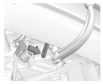
Attach breakaway stopping cable to eye.
