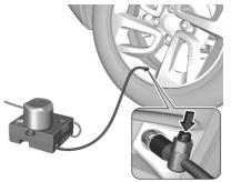
Drain excess tyre pressure with the button on the air hose.
