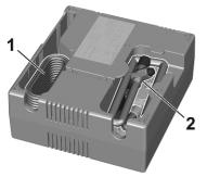
3. Remove the electrical connection cable (1) and air hose (2) from the stowage compartments on the underside of the compressor.
