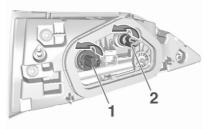
6. Turn the bulb socket anticlockwise and remove it from the light assembly. 7. Detach the bulb from the bulb socket and replace the bulb:
