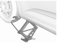
With the jack correctly aligned rotate wheel wrench until wheel is clear of the ground.
