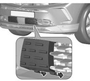
Press the lower part of the protection covers against the slat of the grille. Ensure that the protection covers are fixed securely.
