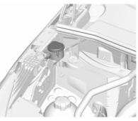
Fill with clean water mixed with a suitable quantity of approved windscreen washer fluid which contains antifreeze.
