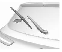
Lift wiper arm. Disengage wiper blade as shown in illustration and remove.
