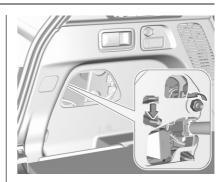
2. Slacken the light fixing nut using a box spanner or socket.
