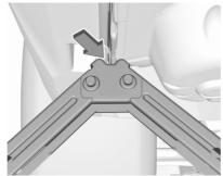
Ensure that the edge of the body fits into the notch of the jack.
