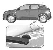
Rear arm position of the lifting platform centrically under the relevant vehicle jacking point.
