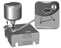
5. Type A: First, insert sealant bottle into the compresor and align the triangle symbols. Then, push down sealant bottle and turn it to the lock position.
