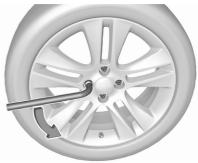
2. Attach the wheel wrench and loosen each wheel bolt by half a turn.
