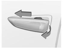
1. Slide the light assembly forward and remove it at the back.
