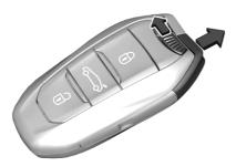
Push the latch to extract the integral key.
