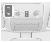
Press button •• or • gently to the first detent: the sunblind is opened or closed as long as the switch is operated.
