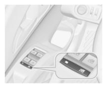
Press switch 🗷 to deactivate rear door power windows, the LED illuminates. To activate, press 🗷 again.
