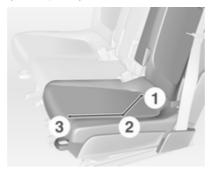
The rear seat row can be adjusted with two seats, providing maximum seating space in position 1, or with three seats in position 2. In position 1 the centre seat is lowered
