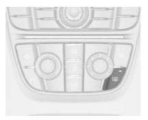
Operated by pressing the button. Heating works with the engine running and is switched off automatically after a short time.
