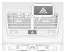
Operated with the ▲ button. Hazard warning flashers ▷ 113.
