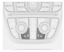
Adjust heating to the desired setting by pressing the #/ button for the respective seat one or more times. The control indicator in the button indicates the setting.
