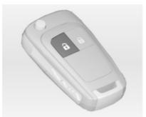
Press button to unlock the doors and load compartment. Open the doors by pulling the handles. To open the tailgate, push the touchpad switch under the tailgate moulding.
