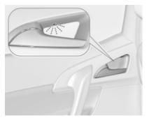
Green LEDs indicate that opening from inside is possible:
