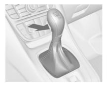
Reverse: with the vehicle stationary, wait 3 seconds after depressing clutch pedal then press the release button on the selector lever and engage the gear.
