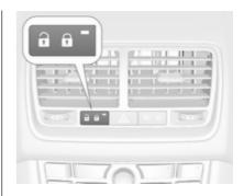
Press central locking button: the doors are locked or unlocked. If the doors are locked, the LED in the button illuminates.
