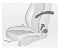
Pull lever, adjust inclination and release lever. Allow the seat to engage audibly.
