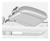
Lower the armrest at the front. Pull the front handle firmly and insert the front guide pins into the upper guide rails. Release the handle. Move the armrest until it engages audibly.
