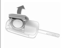
Extend the key and open the unit. Replace the battery (battery type CR 2032), paying attention to the installation position. Close the unit and synchronise.
