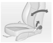
Pull lever, adjust inclination and release lever. Allow the backrest to engage audibly.
