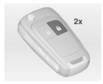
Press on the radio remote control twice within 10 seconds.
