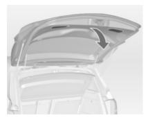
Use one of the interior handles. Do not push the touchpad switch under the moulding whilst closing as this will unlock the tailgate again. Central locking system ♀ 21.
