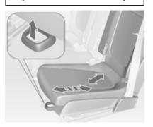
The rear outboard seats can be individually moved forwards or backwards. The seats are movable in longitudinal and transversal directions.
