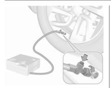
16. Continue driving immediately so that sealant is evenly distributed in the tyre. Drive between 13 mph and 37 mph. After driving approx. 3 miles but no more than 10 minutes, stop and check tyre pressure. Screw compressor air hose directly onto tyre valve when doing this. Fill tyre as described before. Drain excess tyre pressure with the button on the air hose.
