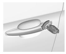
Manually unlock the front door by inserting and turning the key in the lock cylinder.
