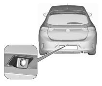
The camera is mounted in the rear bumper above the number plate.
