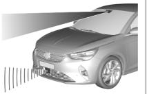
The system uses the front camera in the windscreen and depending on the vehicle configuration a radar unit in the front bumper to detect a pedestrian directly ahead in the path.
