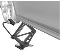
With the jack correctly aligned rotate wheel wrench until wheel is clear of the ground.
