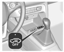
Switch off the monitoring of passenger compartment when animals are being left in the vehicle, because of high volume ultrasonic signals or movements triggering the alarm. Also, switch off when the vehicle is on a ferry or train.
