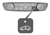
Press Cap to activate the air recirculation mode. The LED in the button illuminates to indicate activation.
