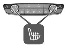
Adjust heating to the desired setting by pressing if for the respective seat one or more times. The control indicator in the button indicates the setting.
