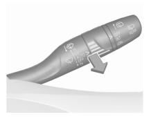
Pull lever. Washer fluid is sprayed onto the windscreen and the wiper wipes a few times. Washer fluid ⇔ 165.
