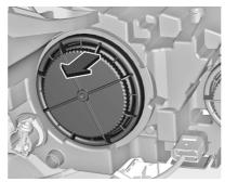
1. Remove the protective cover by pulling.
