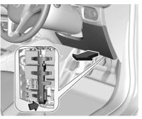
In right-hand drive vehicles, the fuse box is located behind a cover in the instrument panel. Disengage cover at the bottom side and remove. Remove the bracket.
