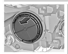
1. Remove the protective cover by pulling.
