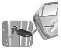
Turn the red child lock in the rear door inwards to the horizontal position by using a key. The door cannot be opened from the inside.
