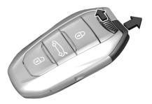
Electronic key: push the latch to extract the integral key.
