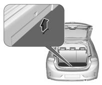
The rear floor cover can be lifted and removed. Use opening to raise the rear floor cover and then remove it.
