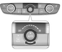
Adjust the air flow by turning rotary ring to the desired speed. Turn anticlockwise to decrease or turn clockwise to increase. Fan speed can also be changed in the climate settings menu. Press **MENU** to enter the menu.
