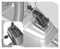
Move the selector lever or press the respective buttons as shown in the illustration above.
