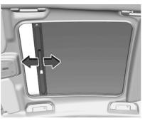
The sunblind is operated manually. Slide the sunblind to the desired position.
