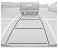
The area behind the vehicle is displayed in the screen. The vertical lines represent the width of the vehicle with mirrors unfolded. The direction of the lines changes with the position of the steering wheel.
