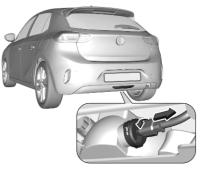
1. Turn the bulb holder anticlockwise and remove it from the reflector housing.
