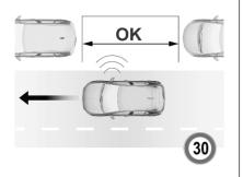
When a free slot is detected, a visual feedback on the Info Display and a first acoustic signal are given. Drive slowly forwards. When the second acoustic signal is given, stop the vehicle, select reverse gear, release the steering wheel and start moving slowly. A visual feedback is given on the Info Display.
