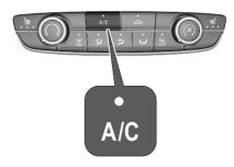
Press **A/C** to switch on cooling. The LED in the button illuminates to indicate activation. Cooling is only functional when the engine is running and fan is switched on.
