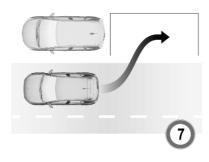
Move forwards and backwards while observing the warnings of the parking assist until the end of manoeuvre is indicated.
