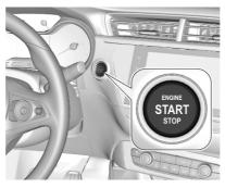
The electronic key or smart access device must be inside the vehicle.
