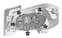
6. Press the five retaining lugs and remove the bulb carrier from the light assembly.
