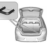
The lashing eyes are designed to secure items against slippage, e.g. using lashing straps or luggage net.
