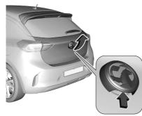
After unlocking, press the tailgate button below the brand emblem and open the tailgate.
