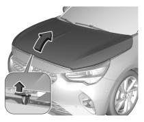
Push the safety catch upwards and open the bonnet.
