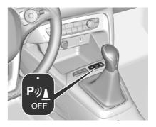
The system is ready to operate when the LED in the parking assist button  $P_{\text{off}}^{\text{wb}}$  is not illuminated. The state of the system is memorised when the ignition is switched off.
