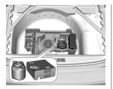
The tyre repair kit is in the load compartment below the floor cover.
