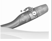
Turn the adjuster wheel to adjust the sensitivity.
