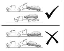
When towing vehicles equipped with an automatic transmission, transport the vehicle on a platform or tow it with the front wheels lifted.
