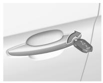
Manually lock the front door by inserting and turning the key in the lock cylinder.
