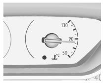
Displays the coolant temperature.
