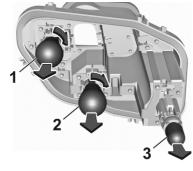
7. Remove and replace the bulbs: Tail light / brake light (1)
