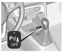
The system is ready to operate when the LED in the parking assist button  $P_{\text{ver}}^{\text{w}}$  is not illuminated. The state of the system is memorised when the ignition is switched off.
