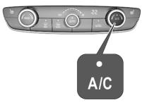
Press **A/C** to switch on cooling. The LED in the button illuminates to indicate activation. Cooling is only functional when the engine is running and climate control fan is switched on.
