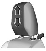
Pull the head restraint upwards or press the catch to release and push the head restraint downwards.
