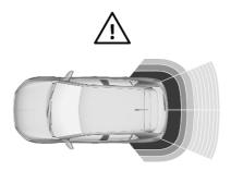
Additionally, the distance to rear obstacles is displayed by changing distance lines in the Info Display ▷ 74. When the obstacle is very close, 介 for danger is displayed.
