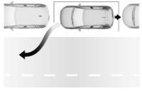
Move forwards and backwards as instructed by observing the warnings of the parking assist and paying attention to the acoustic signals until the end of manoeuvre is indicated.
