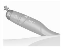
Press **SET / CLR** for 2 seconds to reset the trip odometer. Driver Information Centre  $\Rightarrow$  72.
