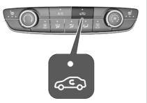
Press Constructed air recirculation mode. The LED in the button illuminates to indicate activation.
