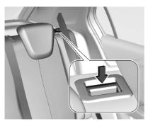
The backrests are properly engaged when the red marks near the release levers are no longer visible.
