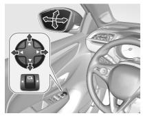
Select the relevant exterior mirror by pushing **A** to the left or right. Then swivel the control to adjust the mirror.
