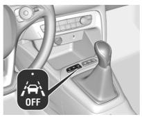
If the system is activated, the LED in the button  $\frac{1}{0F}$  is not illuminated. To activate the system when the system is deactivated, press  $\frac{1}{0F}$ .
