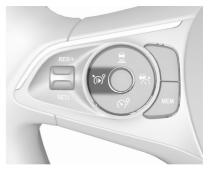
Press  $(\mathbf{b})^{\circ}$ , the adaptive cruise control is in pause mode and a message is displayed. The vehicle is driven without adaptive cruise control.
