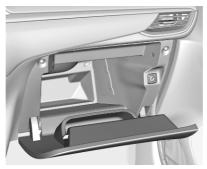
Pull lever to open the glovebox. The glovebox should be closed whilst driving.
