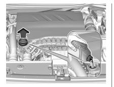
The engine oil level must not exceed the **MAX** mark on the dipstick.
