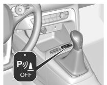
The system is switched off when reverse gear is disengaged. Press  $P_{\text{ver}}^{\text{wa}}$  to deactivate the system manually. The LED in the button illuminates when the system is deactivated. If the system has been deactivated manually, it is not reactivated automatically the next time the ignition is switched on.
