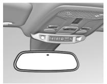
Dazzle from following vehicles is automatically reduced, when driving in the dark.
