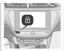
Press **a** to lock. The LED in the button illuminates.
