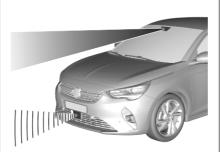
The forward collision alert uses the front camera in the windscreen and depending on the vehicle configuration a radar unit located behind the front bumper to detect a vehicle directly ahead, in the path.
