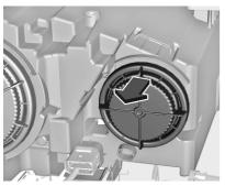
1. Remove the protective cover by pulling.
