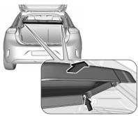
Lift cover at the front and push it upwards at the rear.
