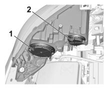
Low beam (1) outer bulb. High beam / daytime running light (2) inner bulb.
