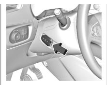
Hold the electronic key at the marking on the steering column cover as shown in the illustration.
