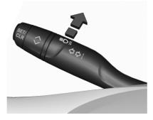
Push to switch from low to high beam. Push again to deactivate high beam. High beam assist ▷ 82.
