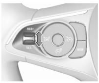
The preset maximum speed can be set by pressing thumb wheel to **RES/+** to increase or **SET/-** to decrease the desired maximum speed. Move thumb wheel repeatedly to change speed in small steps, move and hold to change speed in large steps.
