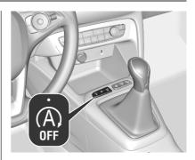
The system is ready to operate when the LED in the button  $\stackrel{\text{\tiny OP}}{\underset{\text{\tiny PP}}{\text{ is not}}}$  is not illuminated. To activate the system when the system is deactivated, press  $\stackrel{\text{\tiny OP}}{\underset{\text{\tiny PP}}{\text{ :}}}$ .
