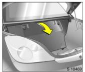
Engage the luggage compartment partition in the rear position. Place no objects in front of the rear window or in front of the luggage compartment partition.
