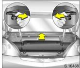
When the Retractable steel roof is closed, the luggage compartment partition can be folded forward to enlarge the luggage compartment.
