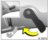
Press the locking levers on upper right and left of the window frame all the way up.
