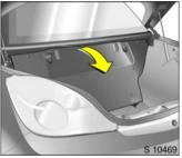
Luggage compartment partition: With the Retractable steel roof closed, pull the centre of the partition, release it and fold it rearward until catches engage.
