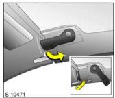
Release the locking levers on upper right and left of the window frame, pulling both levers all the way down. Both retaining hooks must not be engaged.
