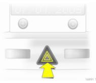
Operated with the  $\triangle$  button. Hazard warning flashers  $\diamondsuit$  111.
