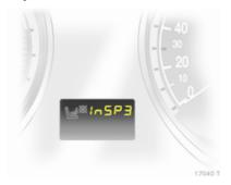
Replace the battery as soon as the system no longer operates properly or the range is reduced. The need for battery replacement is indicated by **InSP3** in the service display or by a check control message in the Info-Display \$\vdots\$ 100.
