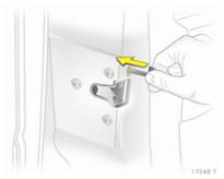
Insert key or emergency key  $\triangleright$  28 into opening above lock on inside of door and operate lock by pressing until it clicks. Then close the door. The procedure must be carried out for each door. The driver's door can also be locked from the outside with the key. The fuel filler flap and tailgate cannot be locked.
