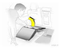
From the load compartment, pull up the seat by the handle.
