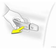
Pull a door handle or press the button under the tailgate moulding.
