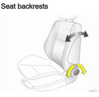
Turn handwheel. Do not lean on seat when adjusting.
