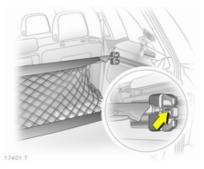
The side walls contain retaining strips, where various components can be attached to divide the load compartment or fasten loads.
