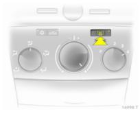
Heating is operated by pressing the III button.
