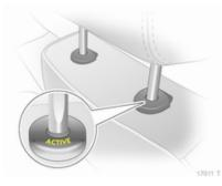
In the event of a rear-end impact, the active head restraints tilt forwards slightly. The head is more effectively supported by the head restraint and the risk of whiplash injury is reduced.
