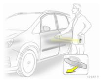
When in possession of the electronic key, simply pulling the door handle will unlock the vehicle and open the door. To open the tailgate, press the button under the moulding.
