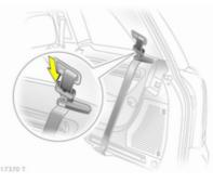
Guide the seat belts through the belt holders and insert the latch plates in the holders.
