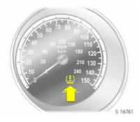
If a tyre loses pressure, it becomes smaller. It then rotates at a different speed than the other tyres. If the system detects a difference in speed, control indicator (1) illuminates red.
