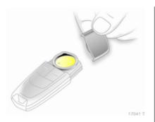
To replace the battery, press the locking mechanism and remove the cap by applying light pressure. Press the cap on the other side outward.
