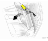
Push the release lever down, adjust inclination, release the lever and engage the backrest.
