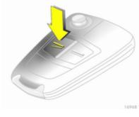
Press button  $\succeq$  to unlock and open door. To open the tailgate, press the button under the moulding. Radio remote control  $\diamondsuit$  27, Central locking system  $\diamondsuit$  31, Load compartment  $\diamondsuit$  34.
