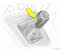
Reverse: with the vehicle stationary, wait 3 seconds after depressing clutch pedal and then press the release button on the selector lever and engage the gear.
