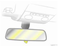
Swivel the lever on the underside to reduce dazzle.
