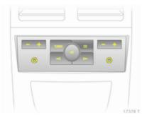
Twin Audio allows occupants in the second row the choice between the audio source played on the infotainment system or a separate audio source.
