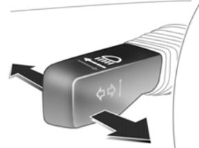
**Headlight flash, high beam and low beam**
