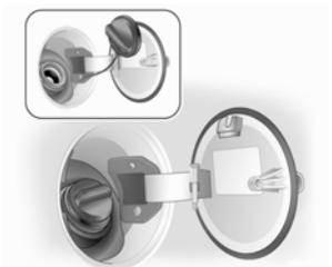
The filler cap can be retained in the bracket on the filler flap.
