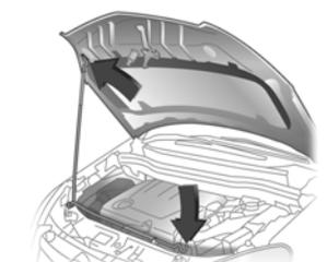
Secure the bonnet in the upright position using the support rod located at the front of the engine compartment.
