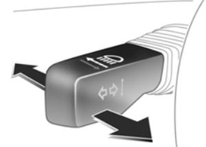
**Headlight flash, high beam and low beam**
