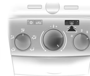
**Heated rear window, heated exterior mirrors:**
