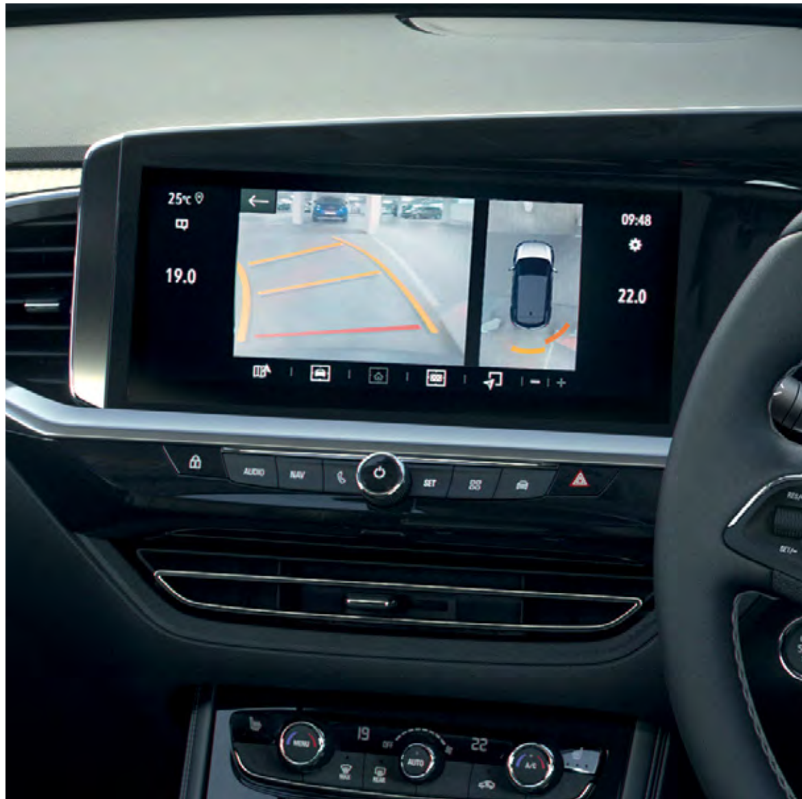
360° Panoramic Parking Camera** This super smart camera gives you a pin-sharp, extra-wide view of the blind spots at the front and back of your car.
