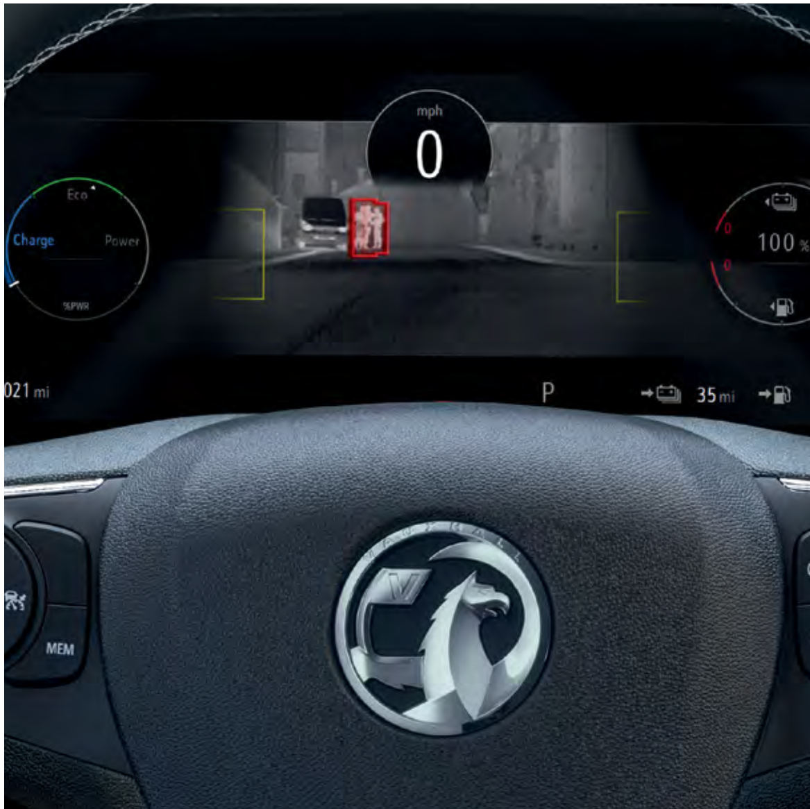
Night Vision Technology* This eye-catching feature can spot pedestrians and animals that stray into the road ahead up to 100 metres away.
