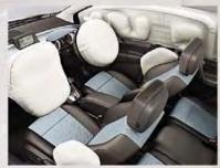
Airbags. Meriva is equipped with front and side-impact airbags for driver and front passenger (front only on Expression models). The front passenger airbag can be deactivated for child seat use. Curtain airbags are also standard on Exclusiv. Tech Line and SE models.
