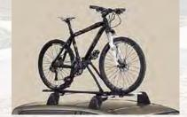
Thule 'Free Ride' bike carrier. Used in conjunction with the Vauxhall base carrier this system allows you to transport a bike on the roof. Supplied with quick release straps and a lock for security.
