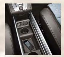
Aux-in socket and USB. Mounted on the centre console, the aux-in socket facility lets you connect your MP3 player (most systems are compatible) to the car's audio system. The USB connection – standard on all models except Expression – allows you to view iPod and memory stick functionality via the audio display.
