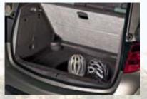
Flex Floor. Our two-position, adjustable luggage compartment floor is standard on all models. When lowered, it maximises rear load height and volume. In the upper position, it's flush with the folded rear seats and the rear sill, providing a flat loadspace area with easy loading – plus a useful 86 litres of loadspace under the Flex Floor.
