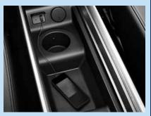
Auxiliary-in socket and USB connection.
