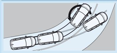
. Electronic Stability Programme-plus (ESP-plus) with Enhanced Understeering Control The system works in conjunction with the car's traction control set-up, sensing when the vehicle is about to slide on a bend and applying corrective braking to the appropriate wheel or wheels, correcting the slide and helping you regain control more rapidly.
