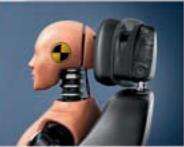
Active-safety front seat head restraints. New Meriva's active front seat head restraints move up and forward under a rear impact to minimise the risk of whiplash injury and guard against other head and upper body injuries. Standard on Exclusiv and SE models, optional as part of the Protection Pack on Expression and S.
