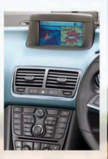
Auxiliary-in and USB. Mounted on the centre console, the auxiliary-in facility lets you connect your MP3 player (most systems are compatible) to the car's audio system. The USB connection – standard on all models except Expression – allows you to view iPod<sup>™</sup> and memory stick functionality via the audio display.
