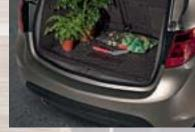
**Semi-rigid cargo liner.** Protect the load area with this semi-rigid moulded plastic liner. Designed with lipped sides for a snug fit, it provides maximum protection, yet is easily removed for cleaning.
