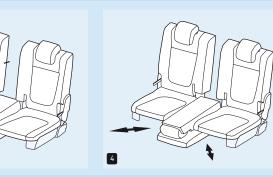
5 Accessible from within the luggage compartment, convenient release straps enable each part of the 40/20/40 rear seat backrest to be folded forward to give a flat load area capable of carrying loads of up to 1642mm in length.
