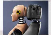
Active-safety front seat head restraints. Meriva's active front seat head restraints move up and forward under a rear impact to minimise the risk of whiplash injury and guard against other head and upper body injuries. Standard on Exclusiv, Tech Line and SE models, optional as part of the Protection Pack on Expression, S and Active.
