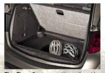
Flex Floor. Our two-position, adjustable luggage compartment floor is standard on all models. When lowered, it maximises rear load height and volume. In the upper position, it's flush with the folded rear seats and the rear sill, providing a flat loadspace area with easy loading – plus a useful 86 litres of loadspace under the Flex Floor.
