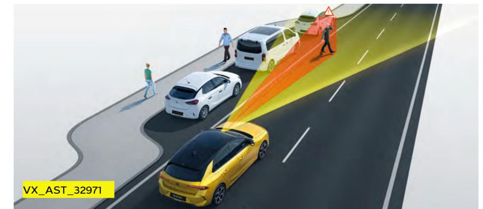
Automatic emergency braking with pedestrian detection.
