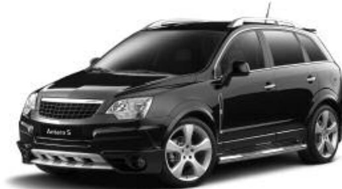
Antara illustrated features Irmischer front lower spoiler, cross hatch grille with aluminium upper, stainless steel door handle covers, side running boards, rear roof spoiler and 20-inch Evo Star alloy wheels.
