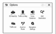
Depending on the former setting, the screen button is labelled **3D Head Up**, **2D Head Up** or **2D North Up**. The map view changes according to the screen button.
