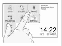
Touch and hold the element you wish to move until red boxes appear around the icons. Move your finger to the desired location and release the element.
