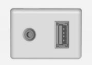
In the centre console below the climate controls, there are an AUX socket and a USB socket for the connection of external audio data sources.
