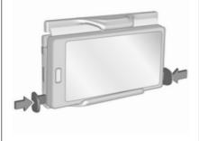
Adjust the width of the phone holder to the width of the phone by pushing together the shifters.
