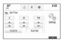
Select **Auto Set** at the bottom of the screen. Activate either **On - RDS** or **Off - Manual**.
