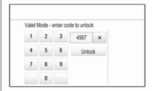
Enter the respective four-digit code and select **Unlock**. The system is unlocked.
