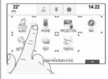
Touch and hold the element you wish to move until frame marks appear around the icons. Move your finger to the desired location and release the element.
