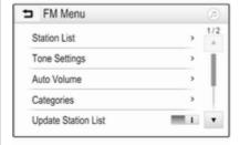
Select the waveband-specific **Station List**. All receivable stations of the relevant waveband and in the current reception area are displayed.
