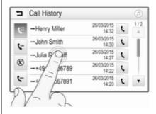
Touch a screen button or menu item. The corresponding system function is activated, a message is shown, or a submenu with further options is displayed.
