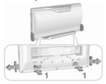
Press both brackets (1) on the rear side to disengage the shifters for width adjustment and pull them out.
