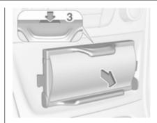
2. Press the release button (3) and remove the phone holder.
