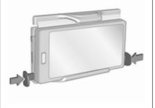
Adjust the width of the phone holder to the width of the phone by pushing the shifters together.
