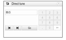
Enter the desired frequency. Use ← to delete digits entered. If necessary, touch I ← or ►I to subsequently adjust the input.
