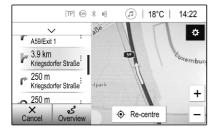
To display a turning manoeuvre on the map, scroll through the list and touch the desired manoeuvre. The map jumps to the respective location on the map. To avoid a route section, select : next to the respective turning manoeuvre. A \* symbol is displayed.
