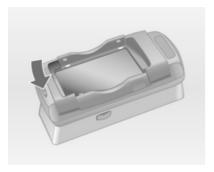
If the side brackets on the adapter are in the closed position, press the button near the front edge of the adapter to open the brackets.
