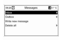
When the mobile phone is paired using the SAP mode, messages can be viewed, composed and sent via the Phone portal. The messages can also be deleted in this menu.
