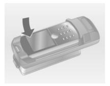
Then lower the top edge. An engaging sound must be audible when the mobile phone engages.
