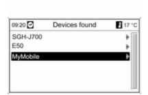
Select the desired mobile phone from the list. The SAP passcode prompt is shown on the Infotainment display containing a 16-digit code.
