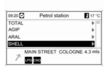
Below the list information on the distance, the direction to follow and the available fuel types (in addition to Petrol and Diesel) is displayed.
