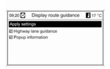
Using the **Popup information** option, it can be determined which type of illustration is to be shown when reaching a highway intersection.
