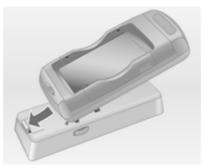
First, lower the front side of the adapter as shown in the above figure.
