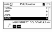
Below the list information on the distance, the direction to follow and the available fuel types (in addition to Petrol and Diesel) is displayed.
