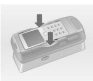
With side brackets of the adapter opened, vertically lower the mobile phone into the adapter as shown in the above figure until the side brackets snap in.
