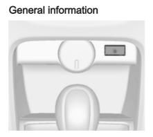
In the centre console there is an AUX socket for the connection of external audio sources.
