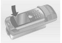
Then lower the top edge. An engaging sound must be audible when the mobile phone engages.
