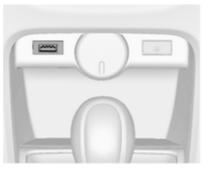
In the centre console there is a USB socket for the connection of external audio sources.
