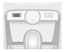
In the centre console there is a USB socket for the connection of external audio data sources.
