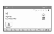
Each waveband has 2 autostore lists (AS 1, AS 2), in each of which 6 stations can be stored.
