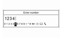
Enter the desired number and select on the display to start dialling.
