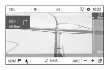
If the autozoom function is activated (AUTO is displayed below the map view), the zoom level changes automatically when approaching a turning manoeuvre during active route guidance. This way, you always get a good overview of the respective manoeuvre.
