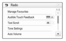
Touch the screen button next to **Audible Touch Feedback** to activate or deactivate the function.
