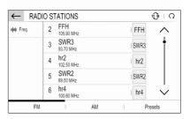
Briefly touch the button next to the desired station. Alternatively, select to switch to the tiled view. Then briefly touch  $Q_{\overline{z}}$  on the tile of the desired station.
