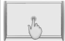
Touch and hold can be used to move an application and to save radio stations on the preset buttons.
