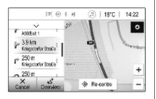
To display a turning manoeuvre on the map, scroll through the list and touch the desired manoeuvre. The map jumps to the respective location on the map. To avoid a route section, select : next to the respective turning manoeuvre. A ♥ symbol is displayed.
