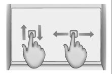
Drag is used to move applications on the homescreen, to scroll through a list or to pan the map. To drag an item, it must be held and moved along the display to the new location.
