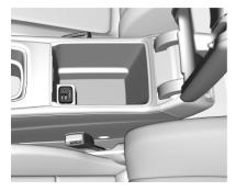
The map data will be delivered on a SD card. The SD card slot is only to be used for navigation map SD cards.
