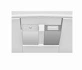
Under the cover on the centre console there is a USB socket for the connection of external audio sources.
