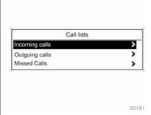
Via the menu **Call lists** the user can view incoming, outgoing and missed calls and dial the relevant numbers. To start a dialling process: select the desired call list, an entry in the call list and finally the desired telephone number.
