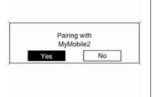
As soon as the Phone portal has detected the mobile phone, the connection set-up can be confirmed.
