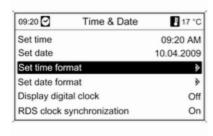
Turn the multifunction knob to move the cursor (= coloured background) to the desired option. Press the multifunction knob to select the marked option.
