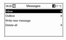
When the mobile phone is paired using the SAP mode, messages can be viewed, composed and sent via the Phone portal. The messages can also be deleted in this menu.
