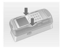
With side brackets of the adapter opened, vertically lower the mobile phone into the adapter as shown in the above figure until the side brackets snap in.
