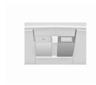
Under the cover on the centre console there is a USB socket for the connection of external audio sources.
