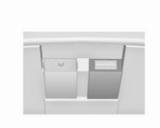
Under the cover on the centre console there is a USB socket for the connection of external audio data sources.
