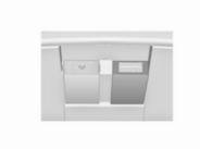
Under the cover on the centre console there is a USB socket for the connection of external audio data sources
