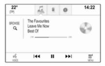
The centre display is located in the middle of the instrument panel. It serves as the main information and control centre of the Infotainment system.
