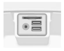
An AUX, USB and SD card socket for the connection of external devices is located underneath the armrest in the centre console. Find a detailed description on lifting the armrest in the Owner's manual.
