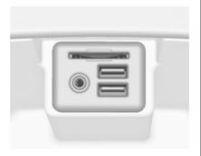
An AUX, USB and SD card socket for the connection of external devices is located underneath the armrest in the centre console. Find a detailed description on lifting the armrest in the Owner's manual.
