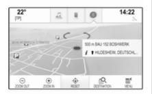
To return to the current location, select the **RESET** screen button in the interaction selector bar.
