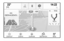
While under active route guidance, select the **DESTINATION** screen button in the interaction selector bar of the map view.
