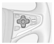
The five-way controller consists of four directional buttons and a confirmation button ( $\checkmark$ ).
