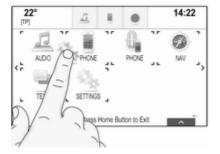
Tap on and hold the element you wish to move until frame marks appear around the icons. Move your finger to the desired location and release the element.
