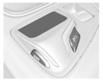
The touch pad has a touch-sensitive surface that allows additional functions for menu control on the centre display. It is located behind the gearshift lever.
