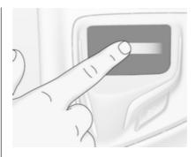
Move your finger in the direction of the element you wish to select. The hand cursor moves from one selectable screen element to the next.
