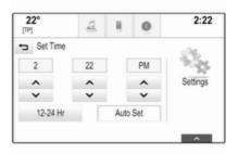
Select the **Auto Set** screen button at the bottom of the screen. Activate either **On - RDS** or **Off - Manual**.
