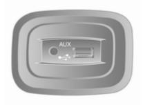
In the Infotainment unit (or in the centre console) there is a USB socket † for the connection of external audio sources.
