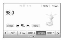
Briefly press or touch I d or → on the control panel or on the screen to play the previous or next station in the station memory.
