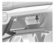
Depending on the version, in the glovebox there is an AUX socket for the connection of external audio sources.
