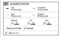
When the menu is opened, several optional routes are automatically calculated by the navigation system, e.g. the fastest route or the most ecological route.
