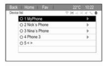
If a new device is paired, it is displayed in the device list.
