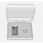
In the centre console there is a USB socket for the connection of external audio data sources.
