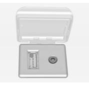
In the centre console there is an AUX socket for the connection of external audio sources.
