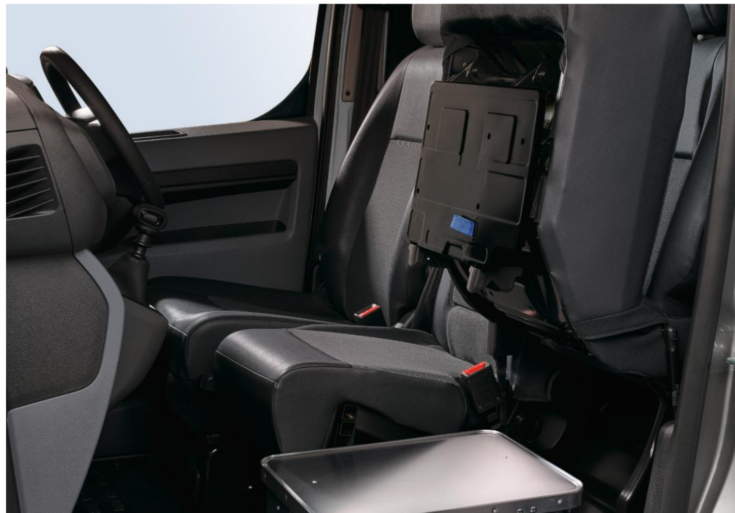
Load-through hatch within bulkhead.
