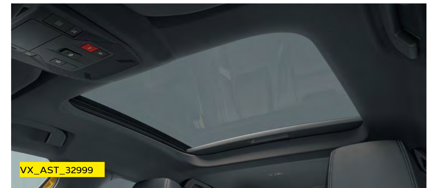
Electrically operated slide/tilt glass sunroof with blind.
