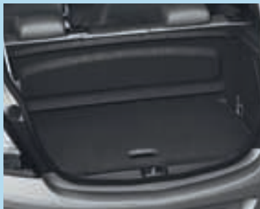
Stowable luggage compartment cover (behind rear seat back) and DualFloor luggage compartment.
