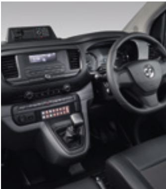
POLICE COMMUNICATIONS RADIO FASCIA AND INTEGRATED 14-WAY SWITCH PANEL.
