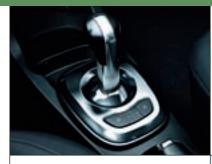
**Easytronic.** Choose Corsa's optional Easytronic transmission and you'll get a fivespeed manual gearbox with a fully automatic mode. In manual mode, you simply push the lever forward or back to shift gears up or down and by nudging the lever to the side you switch to fully automatic mode. There's no clutch pedal so you can drive it on an automatic-only driving licence.
