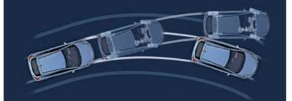
♥ ● Halogen AFL. Another feature you don't expect on a car like Corsa, optional Halogen Adaptive Forward Lighting moves the headlight beams up to 15 degrees left or right of the straight ahead position when you turn the steering wheel, helping improve your vision of the approaching bend.
