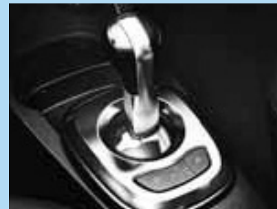
Five-speed Easytronic transmission.
