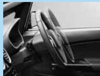
Steering column adjustable for reach and rake.
