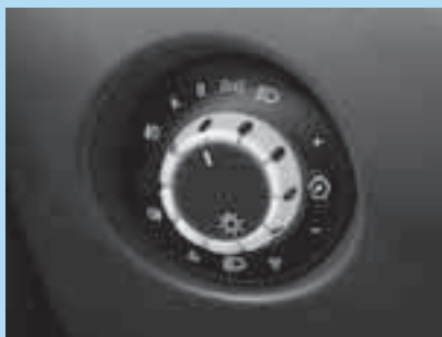
Automatic Lighting Control.
