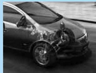
MacPherson strut front suspension.
