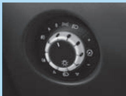
Automatic Lighting Control (ALC).
