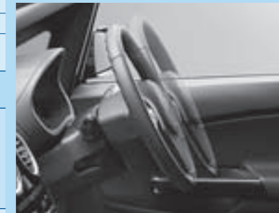
Steering column adjustable for reach and rake.
