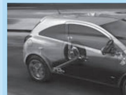
Compound crank rear suspension.
