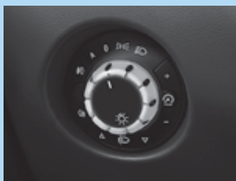
Automatic Lighting Control (ALC).
