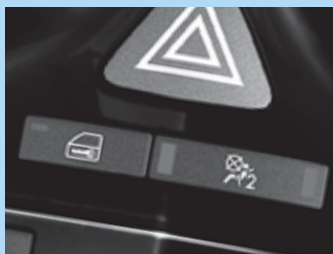
Airbag deactivation and internal door locking switches.
