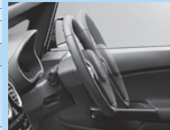
Steering column adjustable for reach and rake.
