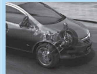
MacPherson strut front suspension.
