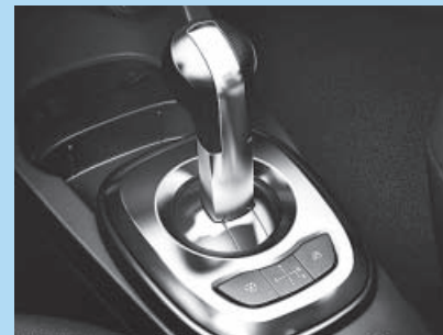
Five-speed Easytronic transmission.
