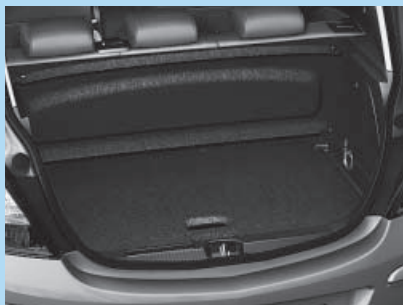
Stowable luggage compartment cover (behind rear seat back) and DualFloor luggage compartment.
