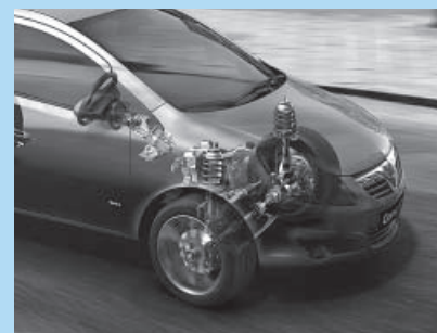
MacPherson strut front suspension.
